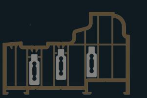
Residence 9 is engineered to meet current and anticipated future standards. Other window frames are typically 3 or 5 chambers and are usually 70mm wide, Residence 9 has 9 chambers and is 100mm wide, resulting in superior thermal, acoustic, strength and security performances.
